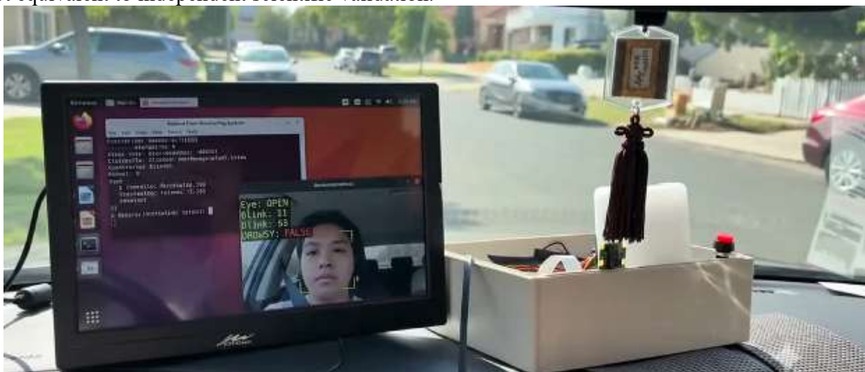
Figure 1. Physical AI Safety Guard prototype demonstrated in a stationary vehicle environment, showing the monitoring display, camera/compute enclosure, actuator housing, and manual control. Source: AI Safety Guard technical presentation, slide 22.
